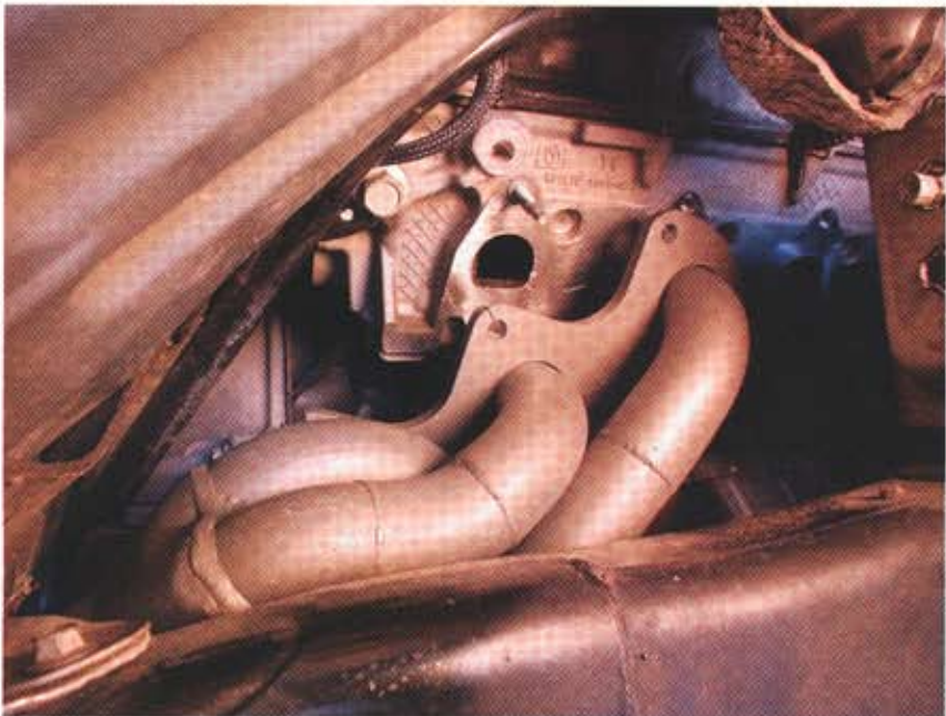
Removing the stock headers and replacing them with the JBA units is the most challenging part of the job.
