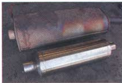
Bigger isn't always better. The larger factory muffler is full of power-robbing baffles.
