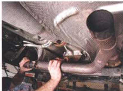
The crossover pipe must be loosened as well.
