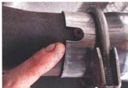
A recess in joints of the JBA tubing ensures that it locks into the proper location.
