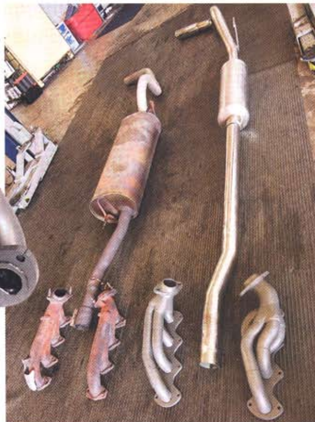
Old versus new: The visual differences between the stock and JBA system really tell the story. Note the differences in the header flanges, tubing, and muffler shape.
