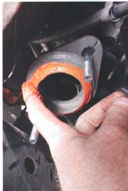
Be sure to add some Ultra Copper high-temp RTV sealant to the collector before bolting on the JBA exhaust pipe.
