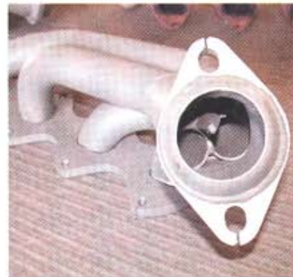
JBA's patented Firecone has a pyramid shape designed to smooth the exhaust flow and maintain velocity for optimum performance.
