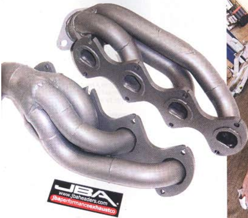
In addition to the Firecone in the merge collector, JBA headers feature thick, laser-cut flanges, over-sized exhaust ports, and smooth, mandrel-bent tubing.
