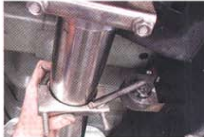
We ran into a bit of difficulty with the hangers, since Ford had made a mid-year change in some of the specs of the stock system. If that's the case with your particular truck, it may take a bit of custom fitting to get the hangers in place.
