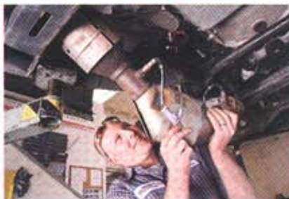
You need to drop down the catalytic converter in order to install the JBA exhaust system.
