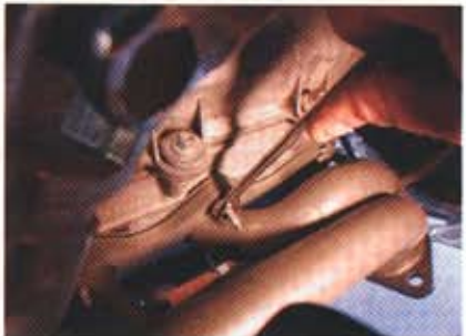
Be prepared to do a few contortions to get at all the header bolts. The clearances around the block can be tight.
