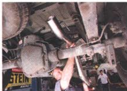
Place the aft end over the rear axle before fitting in the tubing.
