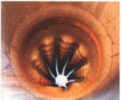
You might think you're staring into the mouth of a python, but it's just a JBA muffler. The scallops cancel out noise without creating excessive flow restrictions.
