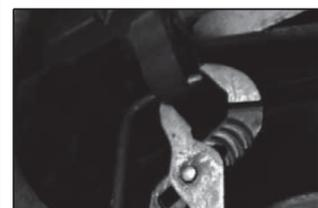
10. Support muffler and remove two rear muffler hangers from rubber grommets using channel lock pliers.
