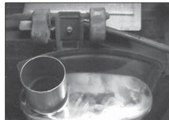
14. Install muffler (B) with offset toward rear and inward.
