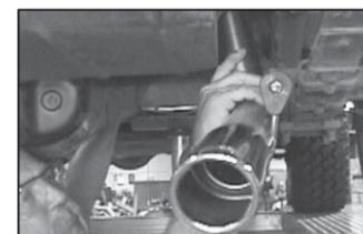
18. Install tail pipe from rear of vehicle. Place rubber grommet in holder and slip tail pipe into rear muffler slip joint 2".
