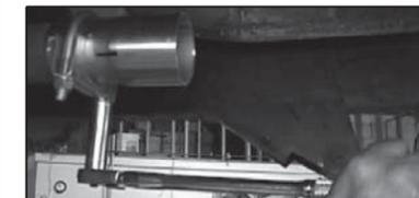
13. Install and position 2" clamp (D), over head pipe (A) slip joint and tighten completely using a 9/16" deep wall socket. NOTE: USE ANTI SEIZE ON THREADS OF CLAMP See notes #3
