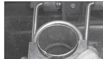
16. Position rear muffler clamp/hanger (F), over rear muffler slip joint and hand tighten only at this time.
