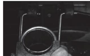
15. Install rear muffler clamp/hanger (F) into lower holes in rubber grommets, with rods pointing toward passenger side.
