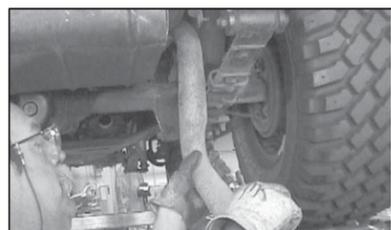
6. Remove tail pipe from rear of vehicle.
