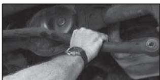
3. With vehicle raised and properly supported, remove pan bar over rear axle by removing two bolts using a 21mm socket or combination wrench and 5/16" allen-wrench.
