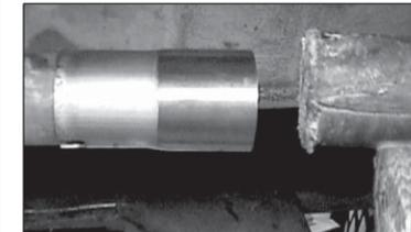
12. Install Evol™ head pipe (A), aligning notch with locating pin. Note: you may have to tap on with rubber mallet. See notes #2
