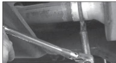
8. Remove front muffler clamp using a 15mm socket.
