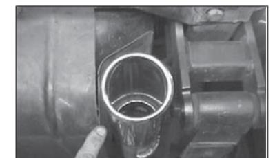
22. Position tail pipe, checking chrome tip for clearance, and tighten clamp/hanger (F) completely using a 9/16" deep wall socket. NOTE: USE ANTI SEIZE ON THREADS OF CLAMP See notes #3
