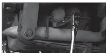
5. Remove rear tail pipe hanger using a 13mm socket and extension.
