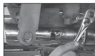
19. Reassemble rear tail pipe hanger assembly, and tighten using a 13mm socket.
