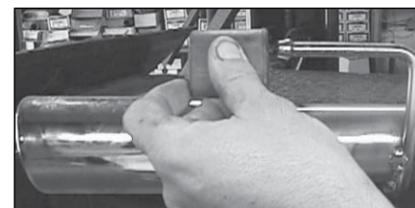
17. Install factory rear tail pipe rubber grommet on rear tail pipe hanger rod.
