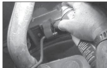
9. Spray lube on two rear muffler hanger rod rubber grommets.
