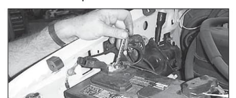
22. Lower vehicle and reattach the negative battery cable.
