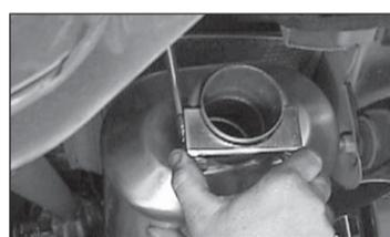
13. Slip clamp/hanger (F) over end of rear muffler slip joint, and hand tighten only at this time. NOTE: USE ANTI SEIZE ON THREADS. See notes #1
