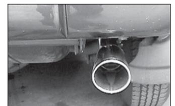
18. Rotate tail pipe (C) to position rear hanger and chrome tip.
