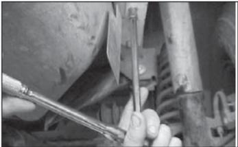
3. With vehicle raised and properly supported, remove tail pipe heat shield by gas tank using a 10mm socket.
