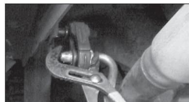
5. Using channel lock pliers, remove tail pipe hanger rod from lower hole in rubber grommet.
