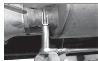
7. Remove front muffler clamp at slip joint, using a 15mm socket.
