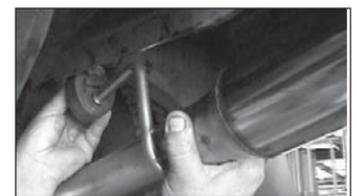
16. Install rear tail pipe hanger rod into lower hole in rubber grommet.
