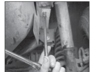
17. Reinstall the tail pipe heat shield using a 10mm socket.
