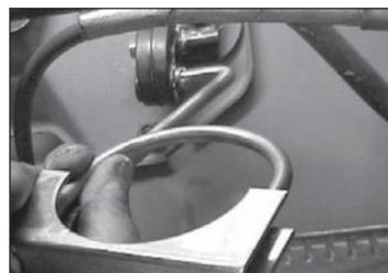
11. With rod pointing toward driver's side, install rear muffler clamp/hanger (F) into lower hole of rubber grommet (G).
