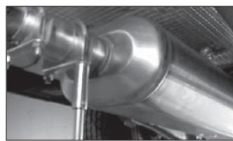
14. Install 2 1/2" clamp (E) over front muffler slip joint. With muffler properly aligned tighten clamp (E) completely using a 9/16" deep wall socket. NOTE: USE ANTI SEIZE ON THREADS. See notes #1
