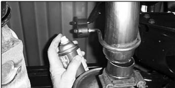
4. Spray lubricant on lower holes of front and rear tail pipe hanger rubber grommets.
