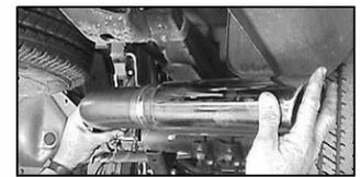
18. Install turn out (D) to end of tail pipe (C) rotate to desired position approx. 1" from body.
