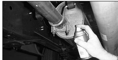
8. Spray penetrating oil on threads of front muffler clamp.
