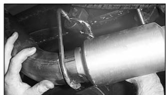
5. Using a pair of channel lock pliers, remove hanger rods from bottom holes of two rear tail pipe rubber grommets.
