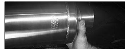
12. With JBA logo facing rear of vehicle, install muffler (B) over head pipe (A) making sure muffler bottoms out on slip joint.
