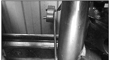
15. Install front two hangers on tail pipe (C) into lower holes of rubber grommet.
