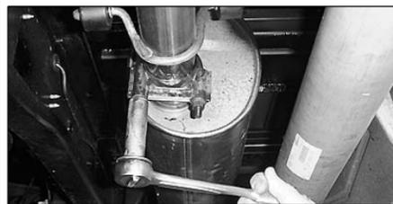
9. Using a 15mm socket, remove front muffler clamp.
