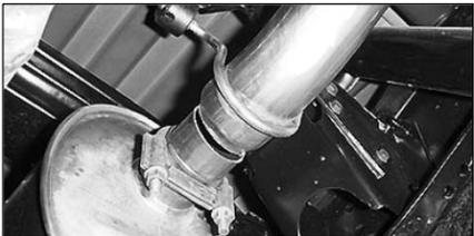
3. With vehicle raised and properly supported, using a reciprocating saw or hack saw, cut tail pipe approximately 1" behind rear muffler clamp and in front of tail pipe hanger.
