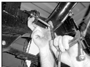
11. Install muffler hanger clamp (E) into rubber isolators near the rear of the factory muffler location.
