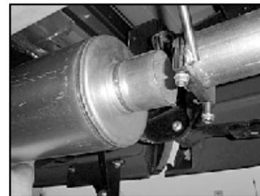
16. Insert tail pipe (C) through muffler hanger clamp (E) and into muffler (B).
