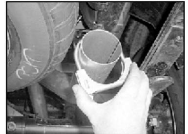
18. Install exhaust clamp (H) loosely over tail pipe (C). Do not tighten at this point.
