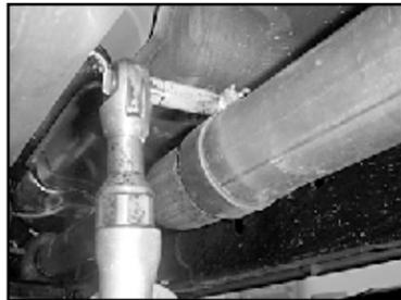
8. Using the 15mm socket and ratchet, loosen the clamp that secures the intermediate pipe to the catalytic converter pipe.
