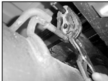
9. Remove muffler hangers from rubber isolators.
