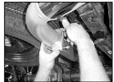
20. Position exhaust clamp (H) over exhaust tip (D).
