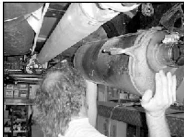
10. Remove factory muffler assembly.
