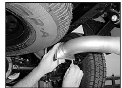
18. Install a standard exhaust clamp (F) where the over axle pipe (C) and tail pipe (D) meet. Secure.
