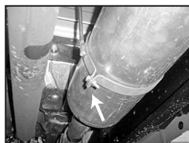
15. Tighten muffler hanger clamp (E) bolt (arrow).
