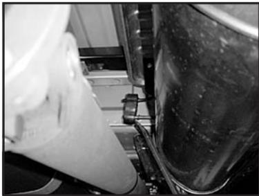
3. With the vehicle raised and properly supported, spray lubricant on all rubber isolators. Using the pry bar, remove rubber isolators from muffler hangers.
