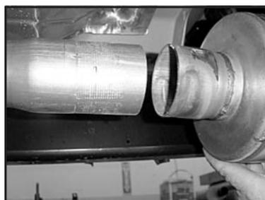
10. Slip muffler (B) into intermediate pipe (A). Install standard exhaust clamp (F) and secure.
