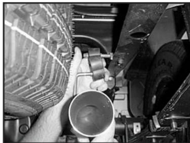
13. Insert rear over axle pipe hanger into factory rubber isolator.
