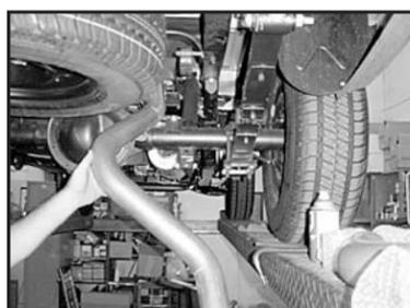
11. Install over axle pipe (C) through the rear of the vehicle.
