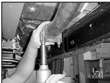
4. Remove the factory exhaust clamp located directly behind the catalytic converter.
