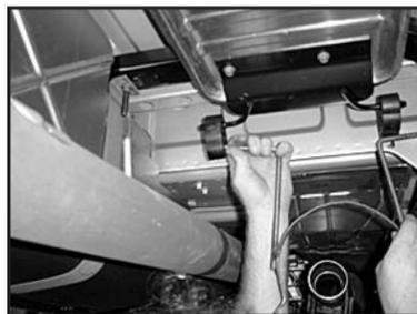
8. Insert hangers on muffler hanger clamp (E) into factory rubber isolators.
