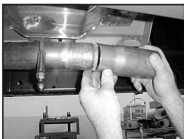
7. Install Intermediate pipe (A). Position pipe properly and secure using standard exhaust clamp (F).
