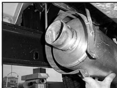
9. Slide muffler (B) through muffler hanger clamp (E). **Note:** install bolt for muffler hanger clamp (E) but do not tighten at this point.
