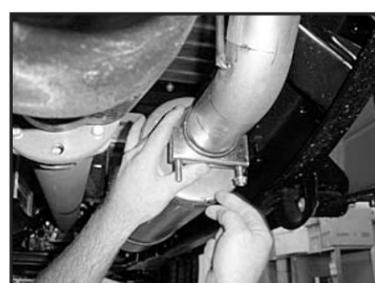
16. Install a standard exhaust clamp (F) at the rear of muffler (B).
