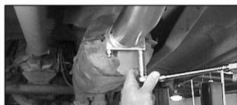
12. Install 2-1/2" clamp (E) on front portion of head pipe (A). Tighten completely with 9/16" deep socket. NOTE: Use anti-seize on threads.
