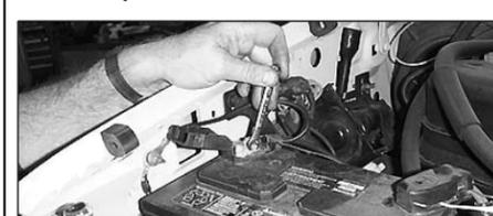
24. Lower vehicle and reattach the negative battery cable.
