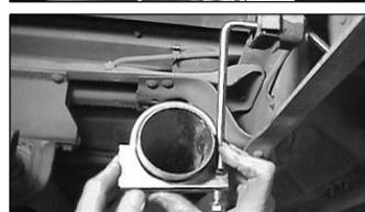
13. Install 3" clamp/hanger (F) into front muffler hanger rubber grommet and position clamp over end of end of head pipe (A).
