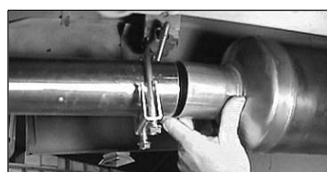
14. Install muffler (B) over head pipe (A) with JBA logo towards rear of vehicle making sure muffler bottoms out on slip joint.
