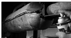
7. Spray penetrating lubricant on front head pipe clamp threads at rear of converter and remove using a 15mm deep socket.
