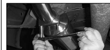
19. Position 3" clamp/hanger (F), level and tighten completely using 9/16" deep socket. NOTE: Use anti-seize on threads.
