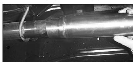
11. Install head pipe (A) aligning notch with locating pin. NOTE: Make sure pin is bottomed out in notch.
