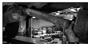
10. Using some form of heat and force, disengage and remove muffler assembly without damaging converter pipe.
