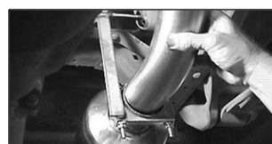
16. Install tail pipe (C) into muffler (B) from rear of vehicle. Longest end towards muffler making sure tail pipe bottoms out in slip joint.
