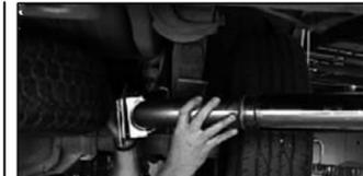
18. Install turn out (D) over end of tail pipe (C) and tighten clamp/hanger (H) lightly with 9/16" wrench. NOTE: Put anti-seize on threads.
