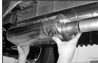
12. Install muffler (B) with offset towards the rear, outside of the truck.
