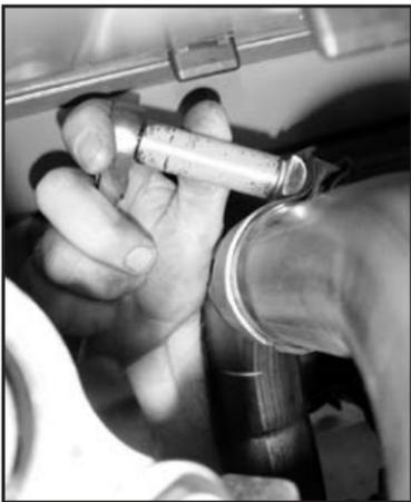
3. With the vehicle raised and properly supported, use a 15mm socket to loosen the clamp on the tailpipe above the axle shaft.
