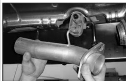
10. Install new intermediate pipe (A).
