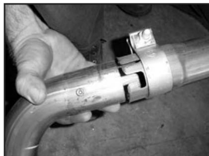
5. The tail pipe attaches by a twist-loc set up. Rotate the tailpipe counter clock wise and pull apart.
