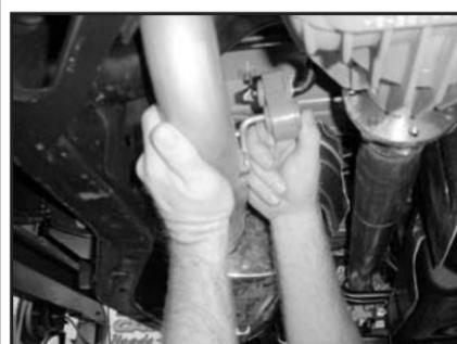
16. Insert forward over axle pipe hanger rod into factory isolator.
