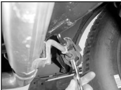
4. Remove the tailpipe hanger from the rubber isolator.
