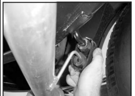
18. Insert tail pipe hanger rod into factory isolator.
