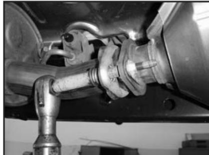
7. Using a 15mm socket, remove the fasteners that attach the exhaust system to the catalytic converter. Save the fasteners, they will be reused.
