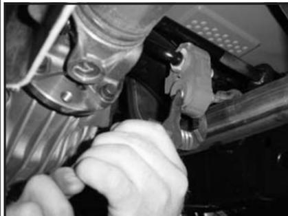
8. Remove factory exhaust system from hangers.
