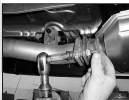
11. Attach new intermediate pipe (A) to catalytic converter by using the original fasteners.
