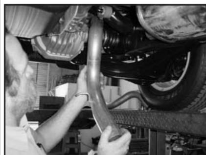
14. Slide rear muffler clamp (G) over muffler outlet. Install over axle pipe (C) with hanger in front of axle.
