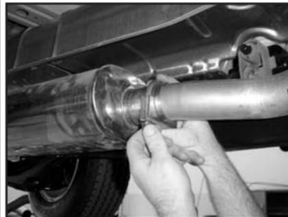
13. Align the muffler (B) and install and tighten front muffler clamp (F).
