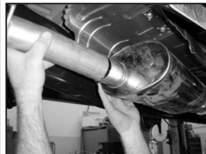
15. Insert over axle pipe (C) into muffler (B).
