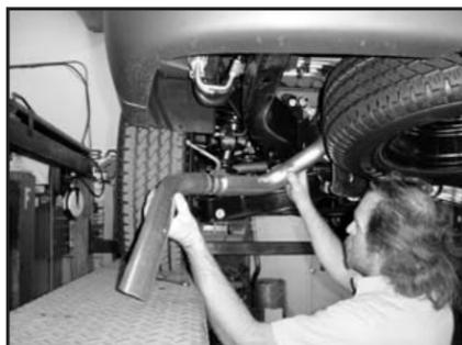
6. Remove tail pipe assembly from rear of vehicle.
