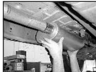
12. Insert muffler (B) into intermediate pipe (A). Install front muffler clamp (E).
