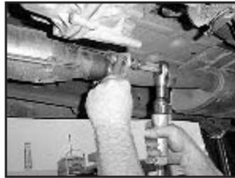
8. Using the 15mm socket, remove fasteners attaching intermediate pipe to catalytic converter.
