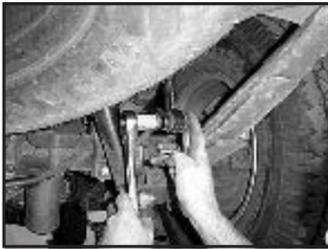
3. With the vehicle raised and properly supported, using the ratchet and the 15mm socket, remove the nut that attaches the sway bar to the sway bar end link on the right side of the vehicle.
