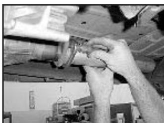
10. Using the factory fasteners, install new intermediate pipe (A).
