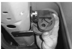
7. Bolt the supplied hanger brackets (H) to the frame on the drivers side using the supplied self tapping screws (J). Bolt the brackets in place with the factory holes. Prongs on the brackets need to face away from each other. Then slide two rubber isolators (G) onto each hanger so holes align.
