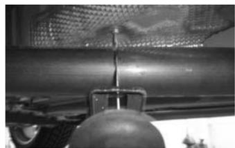
6. Using a reciprocating saw cut the factory h-pipe assembly inline with the heat-shield screw sticking out of the floor on the driver side and passenger side.
