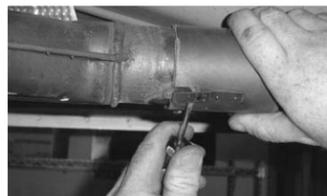
4. Loosen the clamp connecting the exhaust pipe to the muffler. Wiggle the exhaust pipe free from the muffler. Remove the exhaust pipe from car.
