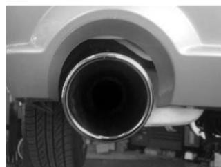
12. With the axle pipes (C) and (D) in the muffler assemblies (E) and (F) adjust mufflers to be flat, and the tips an equal distance from the bumper cover, Then tighten all clamps securely.
