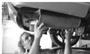
5. Using pliers or a pry bar, slide the rubber hanger from the hanger rod at inside, front of muffler (a little lube helps). Slide the muffler assembly forward and remove from slip hangers.
