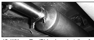
15. With muffler (B) in place, install muffler clamp (E) on slip fit joint. Position 1/4" from lip. Tighten clamp completely with 9/16" deep wall socket. NOTE: Use some anti-seize on all threads.
