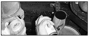
7. Spray lubricant on front and rear muffler hanger grommets.
