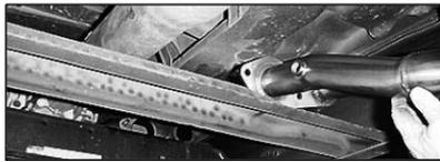
12. Install head pipe (A) with three bolt flange. Install hanger through lower hole in rubber grommet. Tighten three nuts using 15mm socket. Note: we recommend using anti-seize on threads.
