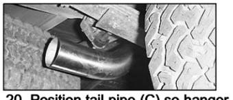
20. Position tail pipe (C) so hanger is not cocked at an angle, and rubber grommet is angled forward.
