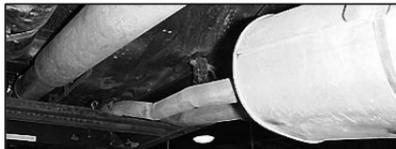
11. Remove muffler assembly pulling towards rear of vehicle. Note: use care not to damage gasket on three bolt flange.
