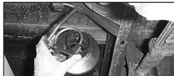
16. Install rear muffler clamp/hanger (F) over slip joint on rear of muffler. Do not tighten at this time.
