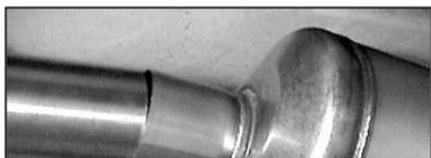
14. Slip muffler (B) on head pipe approximately 2". Note: You may have to tap it in with a rubber mallet. Make sure JBA logo is to the rear.
