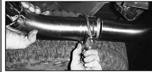
23. Slip turn out clamp (G) onto tail pipe. Slip turn out (D) on tail pipe (C) approx. 1-1/2". Rotate tip to desired position leaving clearance from body. Position clamp (G) with threads in an upward position. Tighten completely with 9/16" deep wall socket. Note: use anti-seize on threads.
