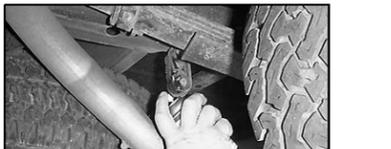
4. Spray lubricant on rear tail pipe hanger grommet.
