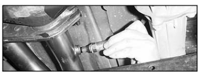
13. Install oxygen sensor using 7/8" wrench.
