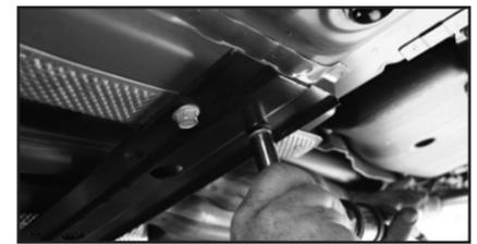
15. With the system tightened and installed to satisfaction, re-install factory cross member.
