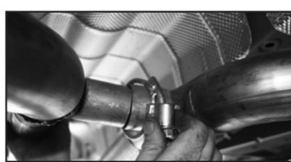
10. Install the intermediate pipes (C & D) by slipping the ends into the H-Pipe assembly. Make sure to position all Sure Seal™ clamps (G) as you build the system.
