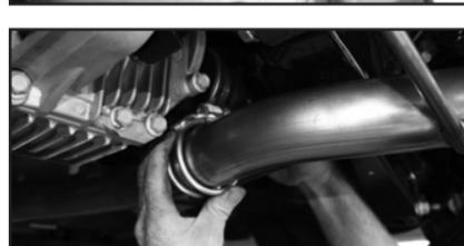
13. Slip the Sure Seal™ clamps (G) over the end of the muffler assemblies and finish hanging them using the factory rubber isolators at the center of the vehicle behind the rear end.
