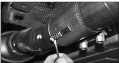
6. Your factory exhaust is a one piece system and it is highly recommended that a second individual be employed to assist in removal. While bracing the factory system, use pliers remove all exhaust hangers from the factory rubber isolators.
