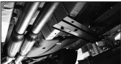
4. Loosen the bolts on both factory band clamps.
