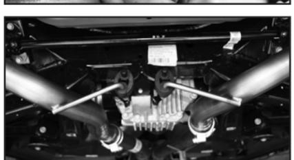
14. Making sure that the tips are centered and positioned well through the rear valence, tighten all clamps.
