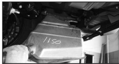
7. With the system free from all mounting points it can be completely removed from the vehicle in one piece.
