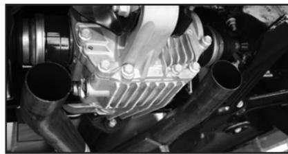
11. With the intermediate pipes in place you are ready to hang the muffler assemblies.
