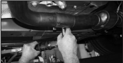
5. Locate the keyways on the band clamps attaching the factory exhaust system to the cat pipe assembly. Using a small flat head screw driver pry the tabs back to release the factory exhaust system.
