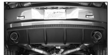
17. Check all clamps and connections for proper fit and alignment. Double check all clamps are tightened and that all hangers are secure in rubber grommets. It is recommended that after installation of the exhaust system you have all slip connections tack welded by a muffler shop.
