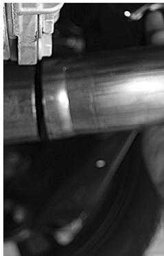
3. Spray WD40 or similar on all bolts and the rubber hangers, remove the rubber hangers from the factory exhaust mufflers. Slide the hangers off the rubber mounts and remove the muffler from the car.
