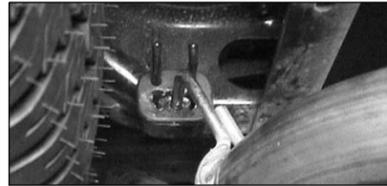
4. Spray lubricant on rear tail pipe hanger rod at lower hole in rubber grommet.
