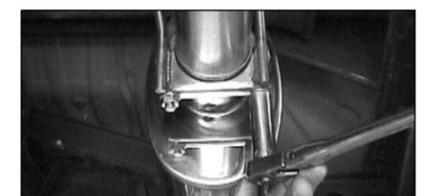
21. Tighten 2-1/2" clamp/hanger (E) completely using a 9/16" socket. NOTE: USE ANTI-SEIZE ON ALL THREADS.
