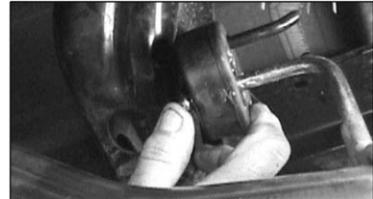
5. Remove rear tail pipe hanger rod from lower hole in rubber grommet.
