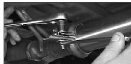
13. Install coupling clamp over flare connection and tighten using a 12mm socket.
