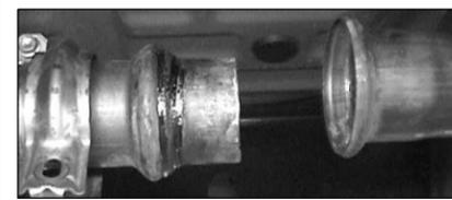
11. Without damaging gasket seal, remove muffler assembly from coupling slip joint.
