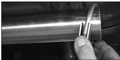
14. Install the 2-1/2" clamp (D) over end of head pipe.
