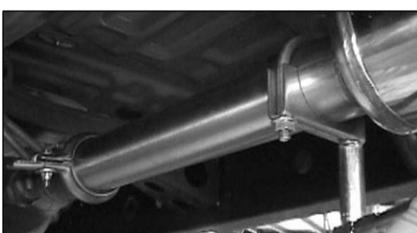
18. Position muffler making sure it is straight up and down. Tighten 2-1/2" clamp (D) completely using a 9/16" socket. NOTE: USE ANTI-SEIZE ON ALL THREADS
