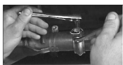
7. Using a 12mm socket, remove bolt from coupling clamp in front of muffler.
