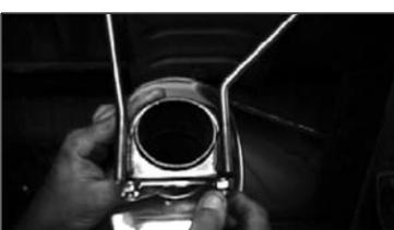
17. Slip rear muffler clamp/hanger (E) over end of muffler (B) rear slip joint and hand tighten only at this time. NOTE: USE ANTI-SEIZE ON ALL THREADS.
