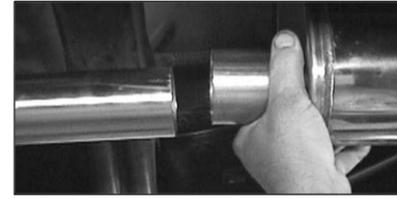
16. Install muffler (B) on head pipe (A) with offset slip joint forward and to the bottom.
