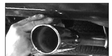
20. Rotate tail pipe to desired position, leaving clearance on rear body panel.
