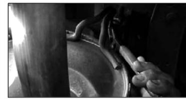
10. With muffler properly supported, remove rear muffler hanger rods from lower holes in rubber grommets using channel lock pliers.
